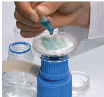
Fig 3. Microbiological media is added to membrane.
