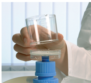
Fig 2. Funnel is removed from monitor unit.
