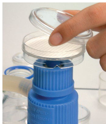
Fig 4. Lid is placed on top of membrane, forming a Petri dish.
