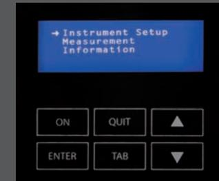
Detail of the 4 lines LCD and the keyboard controls. Unit menu is clearly showed.
