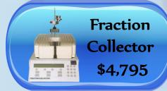
Our fraction collector can be operated as a simple fraction collector, where each fraction is the same size and the fraction size is set in terms of time, drops, or external events (like counts from a pump). A simple command entered from the membrane keypad enables the internal peak detector. This allows you to collect only those peaks of interest from the chromatogram and to ignore the rest.
