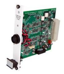
This Amplifier is interchangeable between any of the two BioNex mainframe models. True plug-n-play compatibility allows the user to simply install the card and the software will recognize the module. No hardware / software setup is needed by the user.
