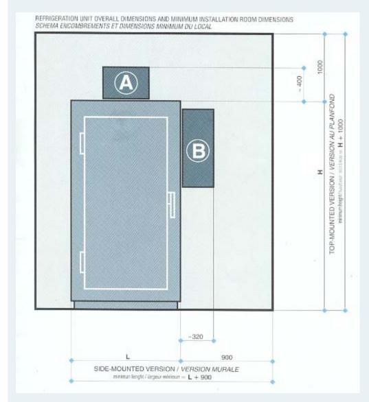
The cooling unit is a single unit containing the condenser, the evaporator and the electronic control panel.
