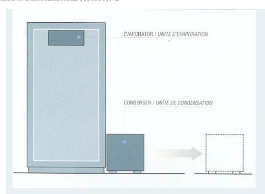
Whenever the space around the refrigeration unit is limited, or whenever the integrated system cannot be used for insufficient aeration in the installation room, it is possible to use the remote system.
