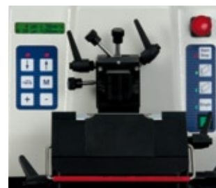
The operating pad for advance / retraction, slow motion, cutting thickness adjustment and trimming
