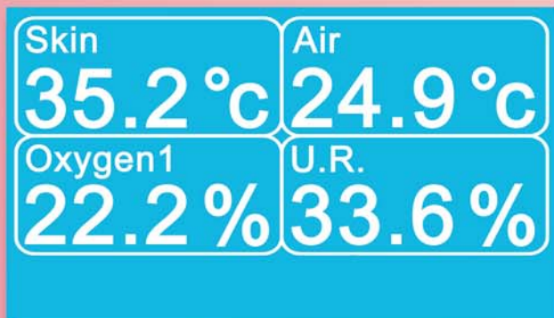
Display for monitoring air and skin temperature, % oxygen and humidity servocontrolled values.
