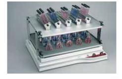
**3019** Analogue Orbital Shaker with Rack Frame 3981, Trays 3980 (2), Test Tube Racks 3953 and Clamps for Erlenmeyer flasks 3983 - 3990
