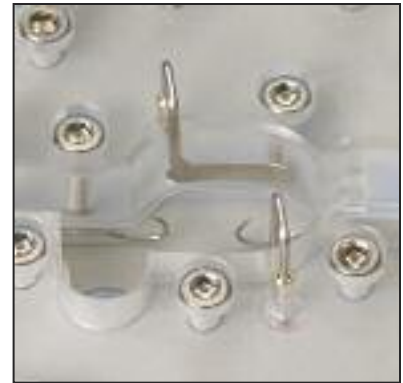
MAYFLOWER Chamber with Field Electrodes
