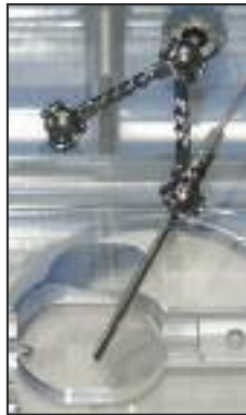
MAYFLOWER Chamber with direct Stimulation Electrode
