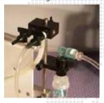
a pre-installed mounting bracket to fit the Dual Diverter Mani-fold (as shown in the picture).
