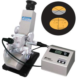
The NAR-1T LIQUID is for liquid sample measurement only. This model has the Refractive Index scale and Brix scale, and operates with D line (589nm) light source. Calibration is performed using distilled water.
