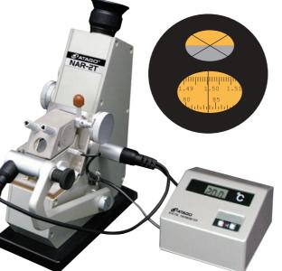
Designed for use with compounds that require measurement at high temperatures (up to 120°C). Capable of measuring samples from 5 to 120°C, such as substances with a melting point higher than room temperature, or compounds containing substances with a transition temperature below 120°C. Aside from liquid samples, glass, films, plastics and other solid samples can also be measured.
