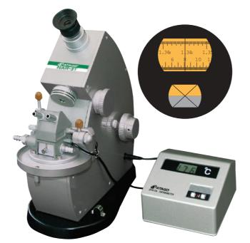
The NAR-3T is the unit with the highest degree of precision and accuracy among the Abbe Refractometers. It was developed to give improved measurement accuracy and ease of use. This was achieved by making fundamental improvements to the optical system and utilizing a larger scale, which allows for a refractive index scale measurements of up to 0.00005. Incorporating a high intensity lamp and using a double control knob gives quick and more accurate control.
