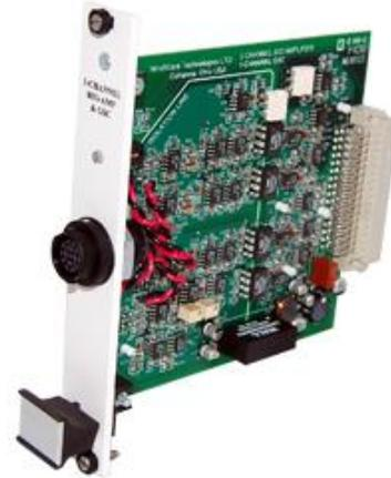
This Amplifier is interchangeable between any of the two BioNex mainframe models. True plug-n-play compatibility allows the user to simply install the card and the software will recognize the module. No hardware / software setup is needed by the user.
