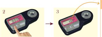
Apply 1 drop of sample solution onto the prism surface.
