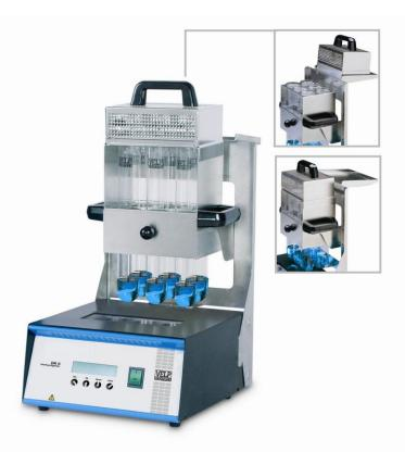
The digester is a widely used instrument in laboratories performing analysis for different applications, such as digestions in the Kjeldahl process for protein determination and analysis in the environmental industry.
