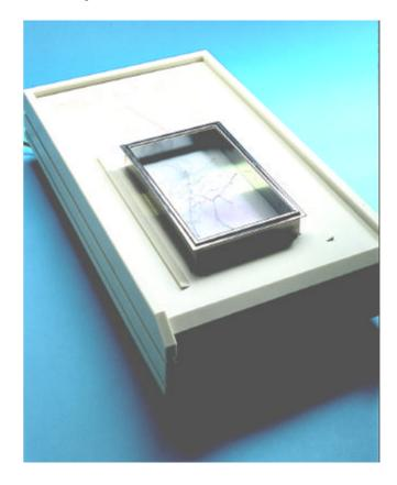
Delta-T Scan offers superior resolution over a much larger area than is possible with systems based on a video camera, and because the scanner delivers digitised images with a precise number of dots per mm, no specific calibration is required.
