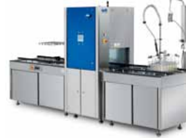
9EWF: In-line continuous Emptying, Washing and Filling station with integrated ERGO series bottle.
