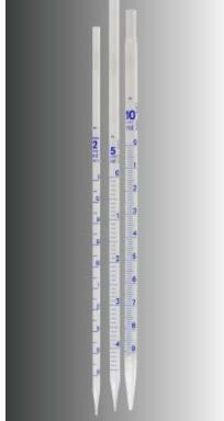
Graduated pipettes, disposable, adjusted EX, tolerance  $\pm 2$  %, serological, made of clear polystyrene, with hydrophobe and coloured cotton plug for rapid identification and perfectly controllable drain, with seamless formed pipette tip to avoid liquid residues, individually packed in paper and plastic, sterile
