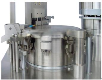
New Design of Fully Enclosed Rotating Table
