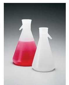
Thermo Scientific Nalgene Polypropylene Flasks with Angled Tubulation are able to withstand vacuum to 30 in. Hg. One-piece for full vacuum service with angled tubulation to prevent tipping.
