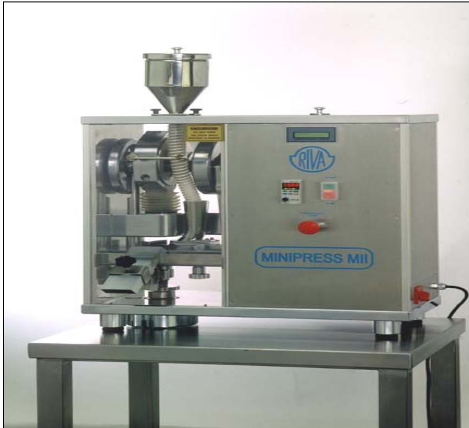
Riva-Minipress , single punch excenter press
