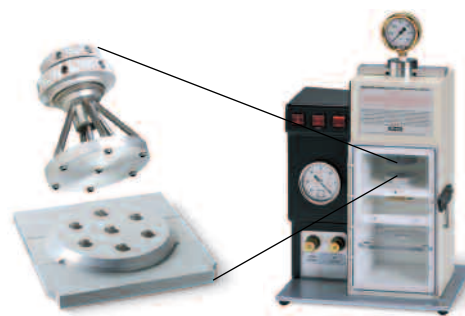
The PDS-1000/He system, shown here with magnified view of the Hepta adaptor.
