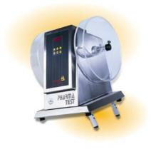
Pharmacopoeia. When finished, the samples have to be de-dusted and weighed again. Actually the difference between the weight before and after the test is determined as friability; which usually should not exceed 1%. Tablets of a diameter more than 13 mm are tested while the instrument is raised on one side by about 10%.
