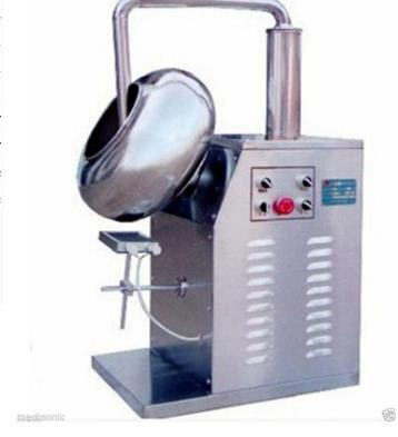
enclosed type, served with airbrush system, and meets the GMP requirements.
