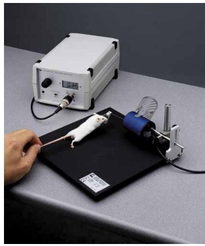
With grasping-BAR, TRAPEZE or GRID TO ASSESS THE FORCE REQUIRED TO MAKE A MOUSE OR A RAT RELEASE GRIP
