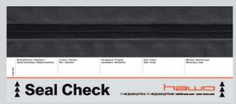
Seal Check An optimum sealing seam is guaranteed when the sealing temperature is correctly set and appropriate to the material to be sealed. Through the daily use of hawotest Seal Check indicators it can be proven that the quality properties recommended by the standards are achieved.
