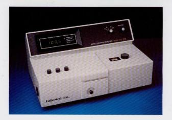
Spectro 22 spectrophotometer is one of the versatile Analytical Instruments used in Conventional Laboratories, which can work in the Visible, Near-Ultraviolet, and Near Infrared Spectral Range, for quantitative and qualitative analysis.
