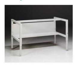
Telescoping Base Stand for use with Purifier® Class II Biosafety Cabinets manufactured since 2000 including the Purifier Delta®, Logic®, Cell Logic®, Logic®+, & Cell Logic®+. Rugged powder coated tube and steel construction. The stand can be installed to provide work surface heights between 30" and 37", in 1" increments. Comes complete with leveling feet
